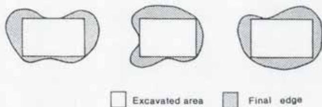
Figure 33. A pond may be excavated in a geometric form, then graded to create a more natural configuration.
